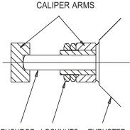
PUSHROD LOCKNUTS THRUSTER
