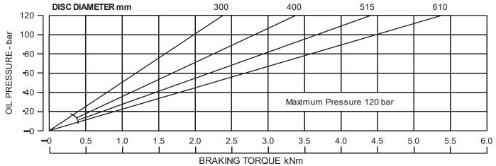
1 kNm = 737.6 lbf-ft 1 bar = 14.5 psi The ratings shown on the above graph are based on fully bedded-in pads. IMPORTANT. This Caliper must only be used with MINERAL OIL BASED HYDRAULIC FLUID.
