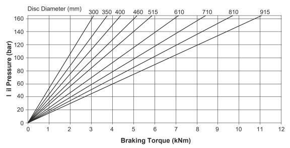
The ratings shown on the above graph are based on fully bedded and conditioned brake pads with nominal friction coefficient  $\mu$ =0.4.
