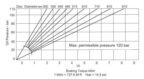
Brake Perfomance of T20 Disc Brake Caliper
