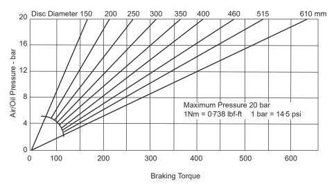
The ratings shown on the above graph are based on fully bedded-in pads.
