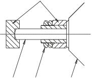
PUSHROD LOCKNUTS THRUSTER
