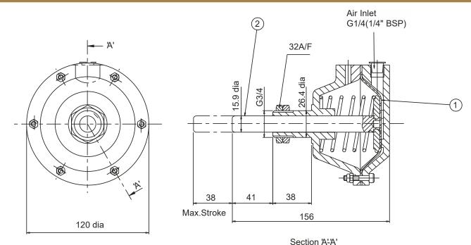
This range of pneumatically operated brakes uses dry and filtered compressed air at pressures up to 7 bar. Pneumatic brakes require a control valve which may be operated either manually, or by pneumatic or electrical signal.
