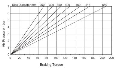
The ratings shown on the above graph are based on fully bedded and conditioned brake pads with nominal friction coefficient  $\mu$ =0.4.
