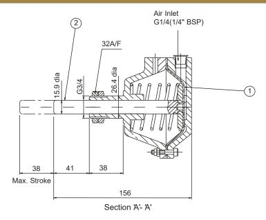
This range of pneumatically operated brakes uses dry and filtered compressed air at pressures up to 7 bar. Pneumatic brakes require a control valve which may be operated either manually, or by pneumatic or electrical signal.
