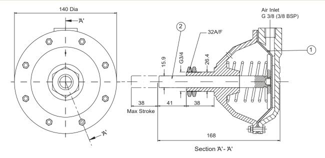
This range of pneumatically operated brakes uses dry and filtered compressed air at pressures up to 7 bar. Pneumatic brakes require a control valve which may be operated either manually, or by pneumatic or electrical signal.
